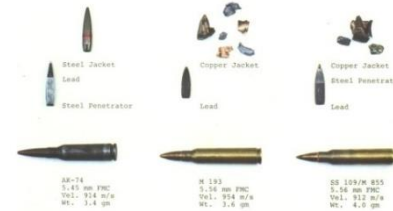
Fig. 14. From bottom to top, the intact round, a cutaway showing the internal construction, and the bullet as it appeared after striking a multi-layer aluminum can shown for a bullet fired from a Soviet AK74 (left), an M16 bullet fired from an M16A1 (middle), and an M855 bullet fired from an M16A2 or an M249 Squad Automatic Weapon (SAR) (right). © 2000 US Army Institute of Research
